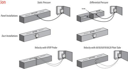
For velocity applications, use the VFXP Series air velocity/measurement probe or AA18, AA19 or AA20 velocity pitot tubes. For use with the PX3P (panel) and PX3U (universal) models in Velocity mode only. Sold separately.
